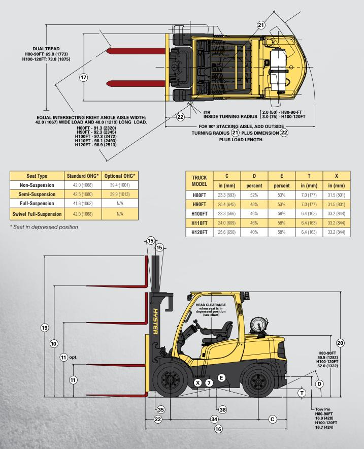
Circled dimensions correspond to the line numbers on the tabulated chart inside the Technical Guide. Dimensions are in inches (millimeters).
